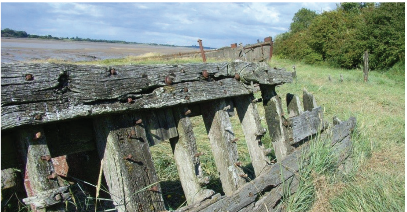
Purton Hulks, River Severn, Gloucestershire. The Purton Hulks are the decayed remains of abandoned boats and ships, deliberately beached in the 1950s to reinforce the banks of the Severn and now interwoven with the landscape. Many of the vessels, including the Severn Collier pictured, were used to transport commodities such as coal along the river and surrounding waterways.
