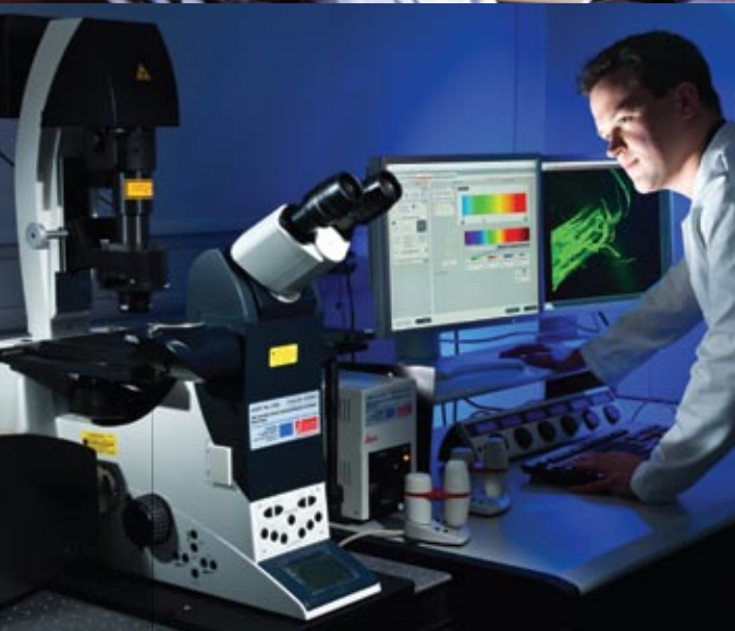
Examining fluorescent markers on plant roots using laser scanning confocal microscopy. ◀ The tunable white light laser enables a wide variety of such markers to be studied
