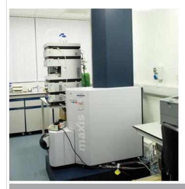
Ultra high resolution - time of flight mass spectrometer (TOF-MS) for use in applications such as: identification of small molecules, metabolomics, quantitative proteomics, biomarker discovery, characterisation of (bio)polymers and supramolecular assemblies.
