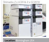
Two HPLC and two GC systems for analysis of molecular materials and nanomaterials.
