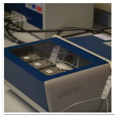
The Quartz Crystal Microbalance provides mass and structural information on molecular layers that form on the surface of a sensor. Molecular adsorption and interactions can be monitored in real time under a variety of conditions. Sensors can be chemically modified to produce a range of surfaces for study.
