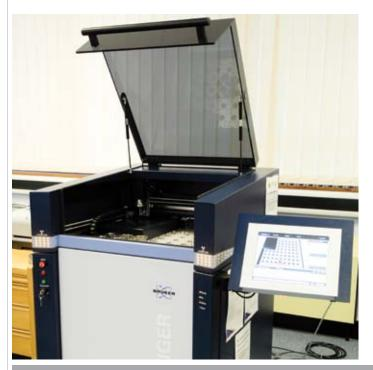
This system is capable of determining the elemental composition of samples, including solids, powders and liquids. It is able to detect elements from oxygen through to uranium.
