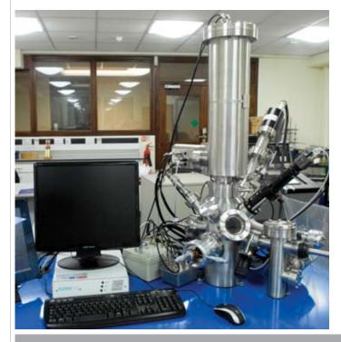
The 'Surface Seer' is a time-of-flight SIMS instrument dedicated to investigating the surface chemistry of materials. A focused caesium ion beam scans an area typically 500 x 500  $\mu$ m on the surface of a sample. This results in mass spectra characteristic of the very top-most atom layers of the sample, which is of increasing importance in materials engineering, biomaterials, drug delivery, etc.
