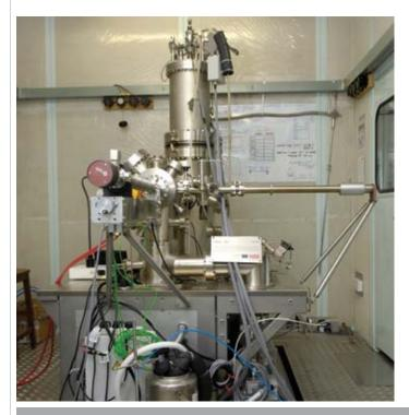
The key to STM is that it can image and probe individual atoms. This allows electronic and vibrational spectroscopy with atomic-scale spatial resolution. They can also image larger areas of surfaces (~ 2 mm<sup>2</sup>) still with high spatial resolution.
