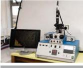
For the thinning of samples such as silicon, ceramics, glass ceramics etc for viewing in the Transmission Electron Microscope.
