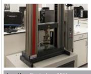
Testing system for compressive and tensile strength of materials.
