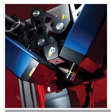
Ellipsometry may be used for the determination of film thickness, morphology, microtribology, electric and optical properties of multilayer metal/metaloxides; self assembled molecules and thin film polymeric materials; next generation energy-efficient glazings. Surface plasmon resonance package is available for molecular surface interaction investigations.
