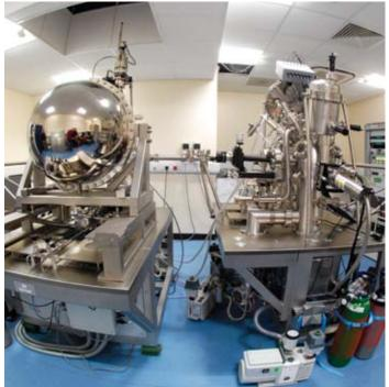
This instrument combines several electron spectroscopy techniques that can be applied to investigate the chemical composition and electronic structure of surfaces and interfaces. The instrument includes a monochromated twin-anode X-ray source (Al & Mg K) and a multi-channel channel concentric hemispherical analyser for high resolution X-ray photoelectron spectroscopy (XPS - supplied by Omicron GmbH).
