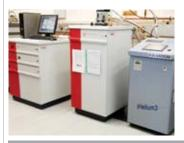
Magnetic Property Measurement System (MPMS) magnetometer utilises Superconducting Quantum Interference Device (SQUID) technology. The MPMS provides solutions for a unique class of sensitive magnetic measurements in key areas such as high-temperature superconductivity, biochemistry, and magnetic recording media.
