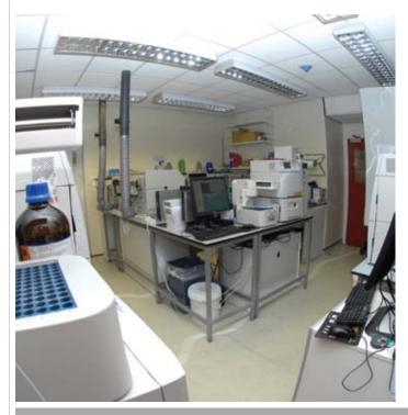
GPC may be used to measure relative molecular weight and polydispersity of polymeric samples.
