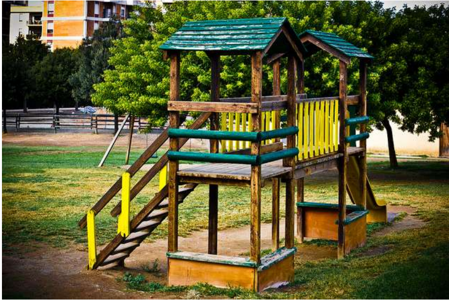
Figure 3. An image affected by vignetting effect. The brightness at the centre of the image is greater than that at the periphery.
