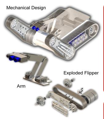
An earthquake scenario presents some very challenging terrain for the robot to navigate; above are some of the CAD designs that satisfy the specific requirements. Currently parts are arriving and designs are being manufactured.
