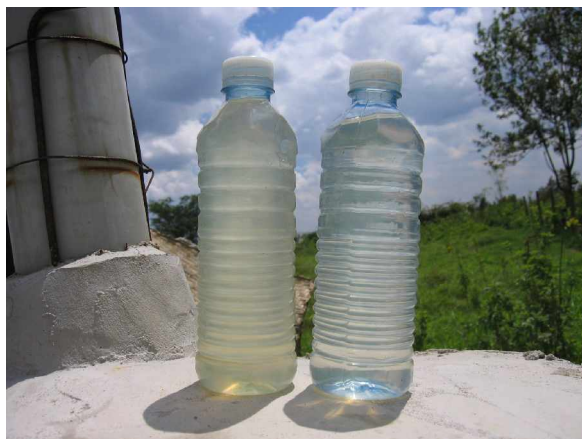
Figure 10 Turbidity reduction in floor filter, input shown on left, output on right.
