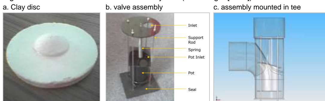
Figure 13.2: First-flush diverter based on clay disc (from Knight [2005])
