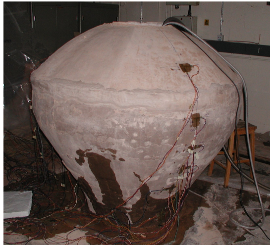
Figure 7.9: External surface of the tank during filling, with dark damp patches indicating locations of leaks
