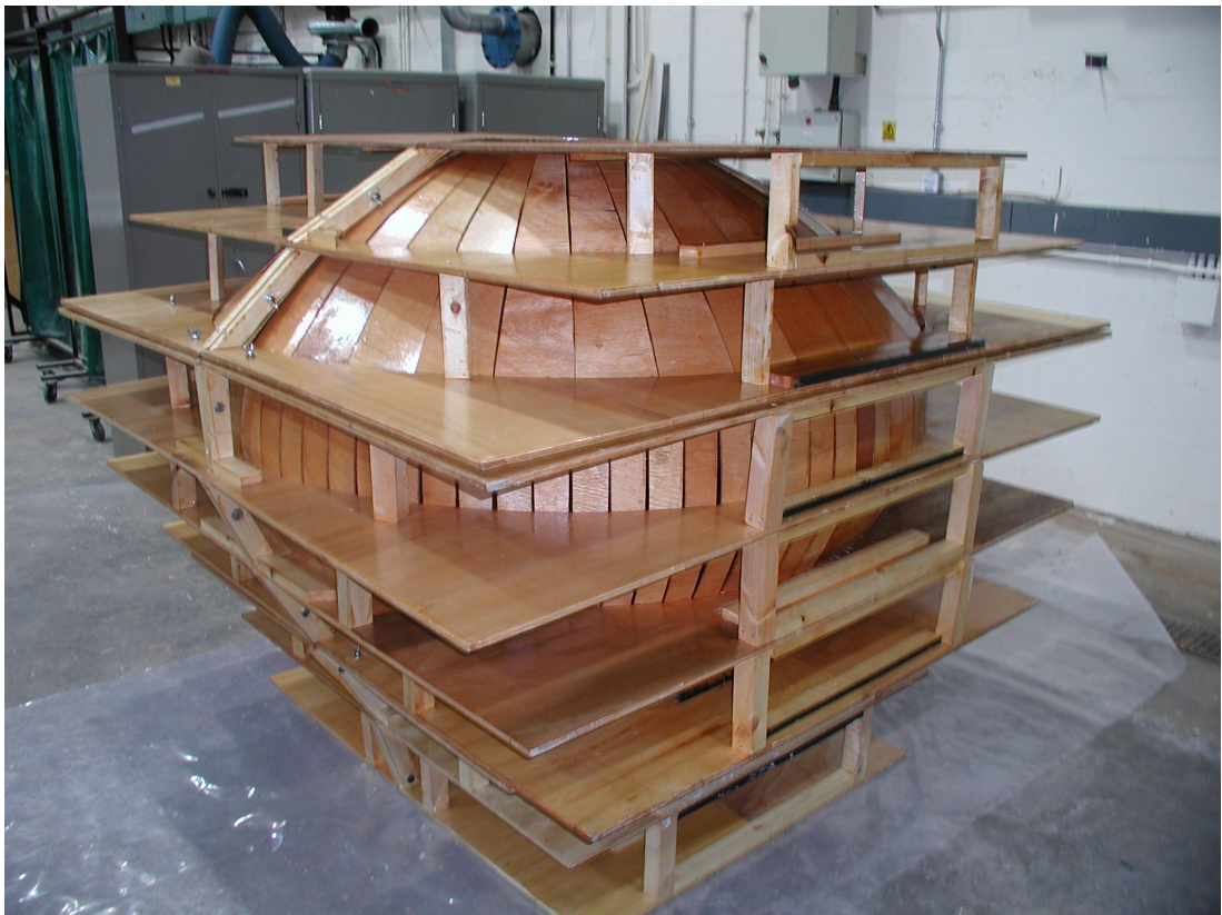
Figure B.6: Assembled frame, with two coats of varnish applied
