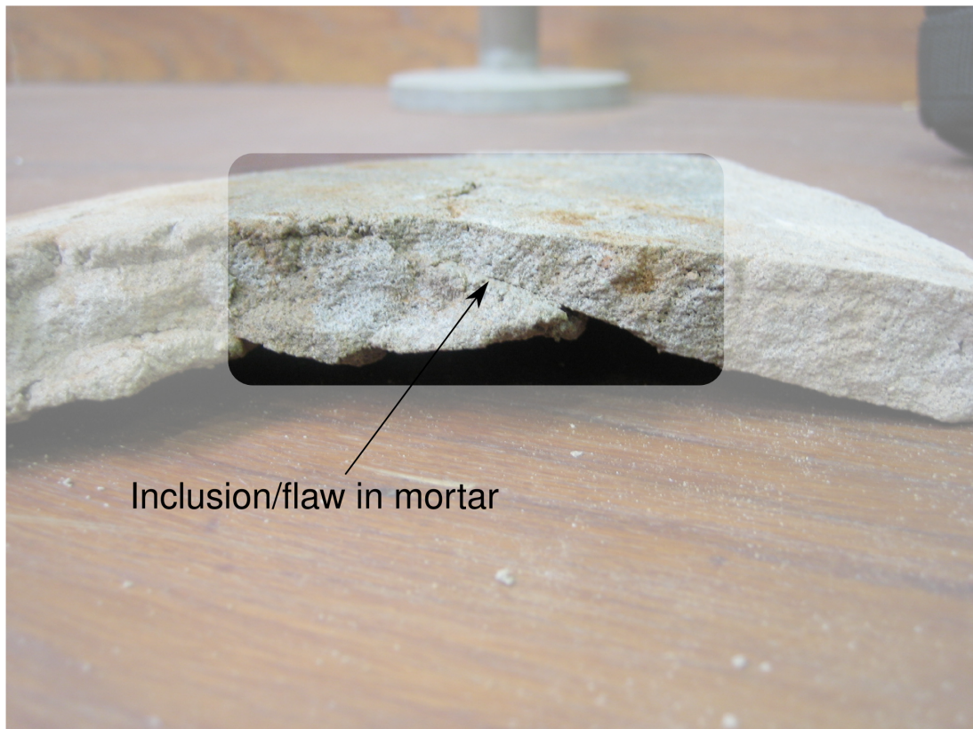
Figure 7.13: Section of the tank, obtained after failure, showing a flaw due to poor plastering during construction
