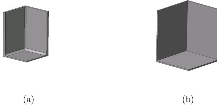
Figure 6.1: Section of 0D curvature tank, with (a), and without (b) radial fillets at panel joints and wall-base joint
