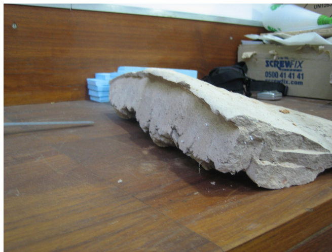
Figure 7.11: Section of prototype tank, indicating clean debonding at joint between lid and lower section of tank
