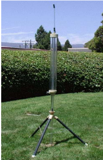
Guelph Permeameter - constant head measurement in the field (after Soilmoisture Equipment Corp. 2008)
