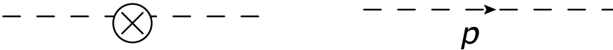
Figure 6.3.1: The new Feynman propagators the one on the left is the counterterm propagator and has associated value i(p^2 \delta_Z - \delta_m) , the one on the right is the normal propagator and by analogue with before has value \frac{i}{p^2 - m^2 + i\epsilon} where m is now the physical mass
