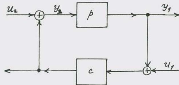
$$H(p, c) := \begin{bmatrix} \frac{-pc}{1-pc} & \frac{p}{1-pc} \\ \frac{-c}{1+pc} & \frac{1}{1+pc} \end{bmatrix} \in R^{2 \times 2}$$
