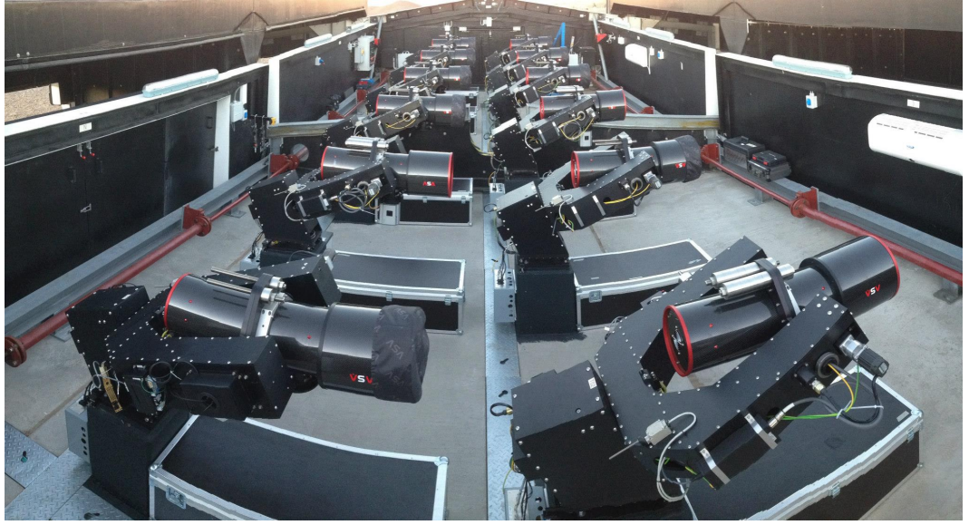
Figure 1.2: The NGTS array of telescopes
