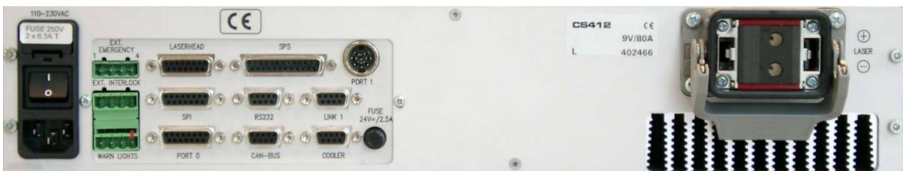
Rear panel CS412 air-cooled, power connector via industrial connector
