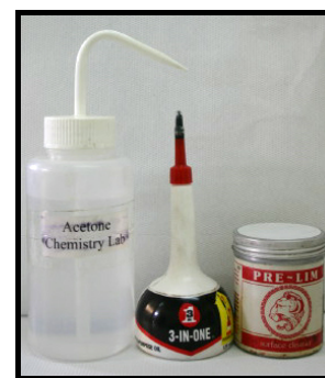
From left: Acetone, 3-in-1 TM machine oil and Pre-Lim TM polishing paste
