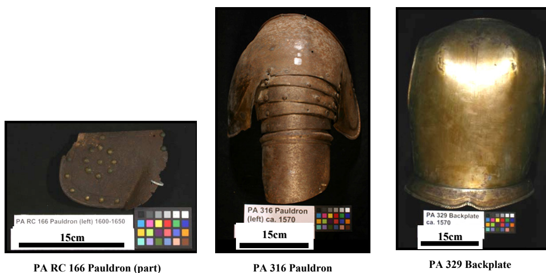
Figure 3-1 The three munition armour accompanying the cross-section samples selected for further laboratory study 823
