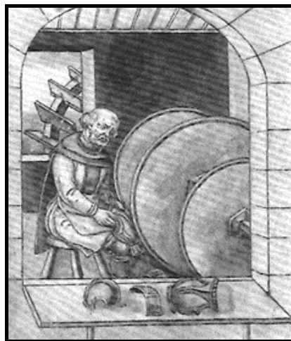
Figure 2-12 An illustration from Hausbuch der Mendelschen Zwölfbrüderstiftung (circa 1571) depicting an armorer using a hydraulic powered polishing/grinding wheel 131
