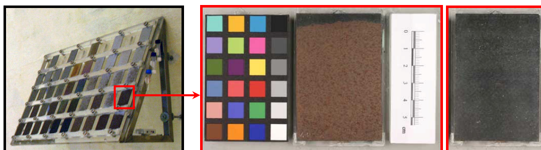
Figure 2-28 Left: Rack containing low-carbon steel coupons exposed at an inclination of 30° to the vertical in the Palace Armoury, Armour Hall 371 . Centre: Very corroded particle-collecting upper side of unprotected coupon after 17 months exposure 372 . Right: Slightly corroded inverted side of corresponding unprotected coupon, which is collecting less particles 373 .
