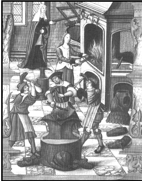
Figure 2-10 A 15-16 th French manuscript depicting hot forming of a breastplate or backplate by hammer on an anvil 120
