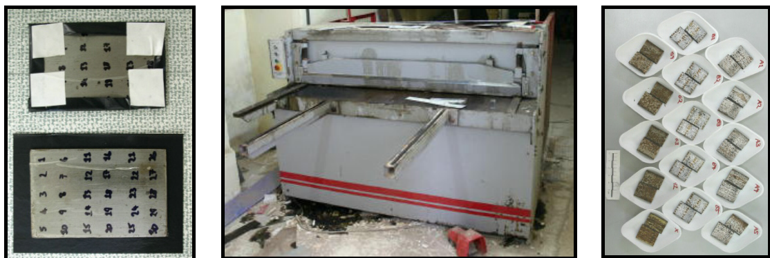
Figure 3-22 Left: Armour analogues being wrapped (bottom: unwrapped, top: wrapped) in carbon paper before cutting. Centre: Industrial sheet metal cutting guillotine used to divide armour analogues. Right: Assembly of cut major-coupons (Armour analogue objective 1, Limitos determination only) from Coupon Series 1, 4 & 6
