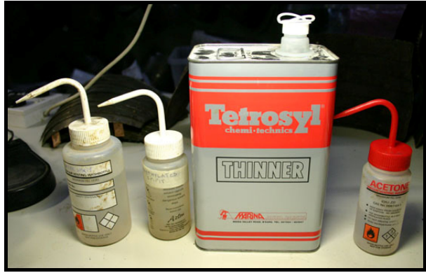
From left: White spirit, methylated spirits, commercial thinner (mixture of aromatic hydrocarbons), acetone
