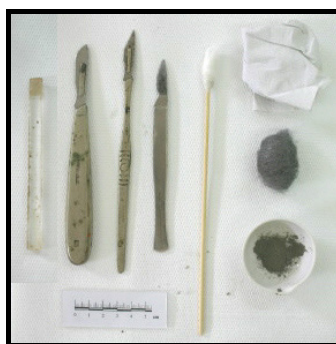
From left and top: Acrylic scraper, scalpels, cotton swab, paper tissue, steel wool and rottenstone powder
