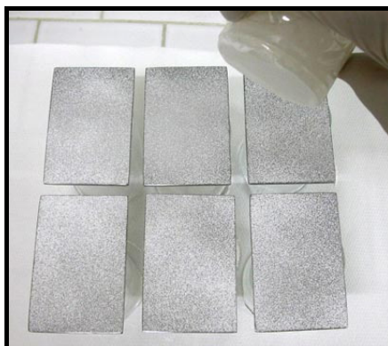
Figure 3-14 Application of zinc oxide/barium sulphate applied superior limitos marker to armour analogue Coupon Series 5
