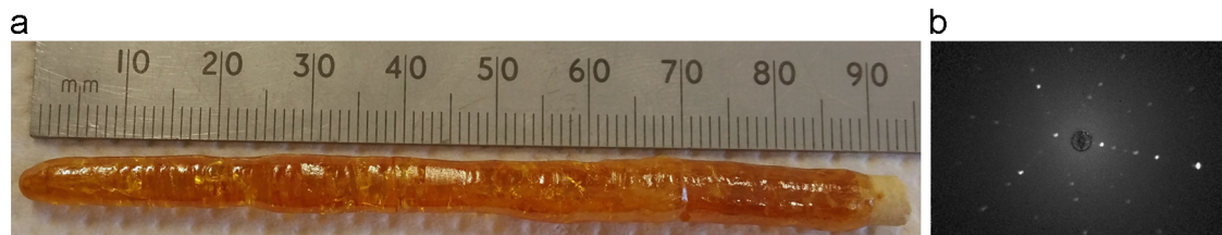
Fig. 5. (a) Boule of \text{Sm}_2\text{Zr}_2\text{O}_7 prepared in oxygen, at 4 bars pressure and using a growth rate of 8 mm/h. (b) X-ray Laue back reflection photograph taken for one of the facets of a \text{Sm}_2\text{Zr}_2\text{O}_7 crystal.
