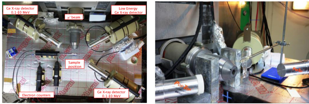
Fig. 5. Photographs of the experiment setup. The picture on the left is the view from above and the picture on the right is from the side. The aerial picture shows the layout and angles of the detectors to the sample. The side view shows a sample being held in place.
