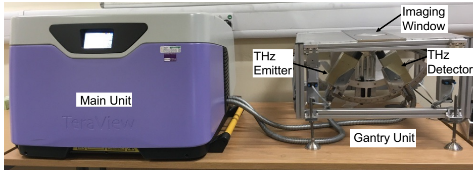
Figure 2.10: The TeraPulse 4000 spectrometer used to perform measurements, showing the main unit and the gantry system used for reflection geometry measurements.
