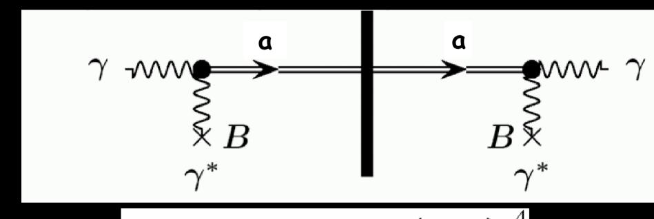
$$P_{\gamma \to a \to \gamma} \sim N_{\text{pass}} \left(\frac{BL}{M}\right)^4$$
