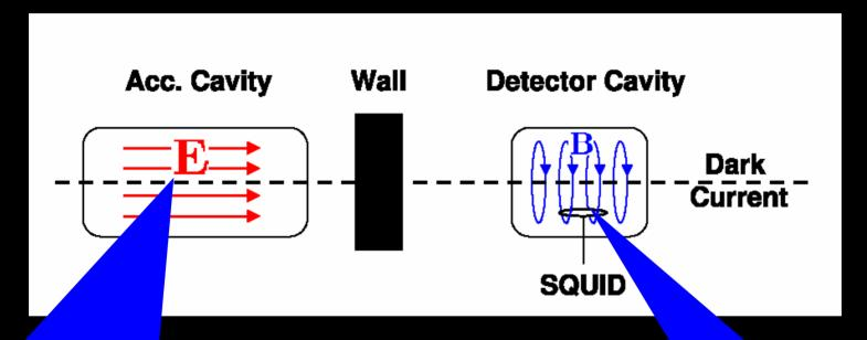
Minicharged particles produced in the cavity lead to a Dark Current
