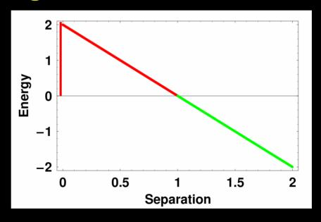
· An f,  $\bar{f}$  -pair separated by a distance  $d > \frac{2}{3}$  has less energy than no particles!
