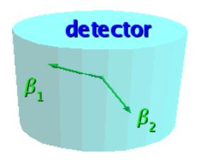
$$T_{1/2} \propto \varepsilon \frac{a}{A} \sqrt{\frac{M \times t}{\Delta E \times B}}$$
