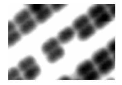
Atomic resolution STM of InAs(001)-(2x4)showing arsenic dimer-pair-rows, missing dimer defect and unit mesh registry defect. Image ~ 4.5 by 3 nm. As dimers have high LDOS at negative sample bias... 'filled states' image.
