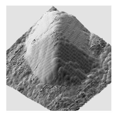
3D rendering of STM image of single InAs quantum dot on GaAs(001), showing atomic resolution on the dot sides. SPM techniques give a true 3D topography – e.g. one can integrate to get the volume.
