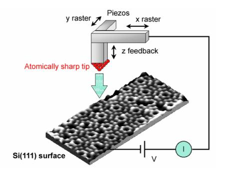
Constant current mode: keep tunnelling current constant by adjusting z with feedback system as x and y are rastered  $\rightarrow$  image made up of (x,y,z) coordinates, contrast via topography and LDOS.
