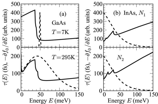
FIG. 1. (a) Calculated dependence of the scattering time  $\tau$  (solid lines) and  $-\partial f_0/\partial E$  (dashed lines) upon the electron energy  $E$  for GaAs at  $T = 7 \text{ K}$  and  $T = 295 \text{ K}$ , with  $N = 9 \times 10^{17} \text{ cm}^{-3}$ . (b) As (a), but for InAs at room temperature at electron densities  $N_1 = 1.4 \times 10^{16} \text{ cm}^{-3}$  and  $N_2 = 3.9 \times 10^{16} \text{ cm}^{-3}$ .
