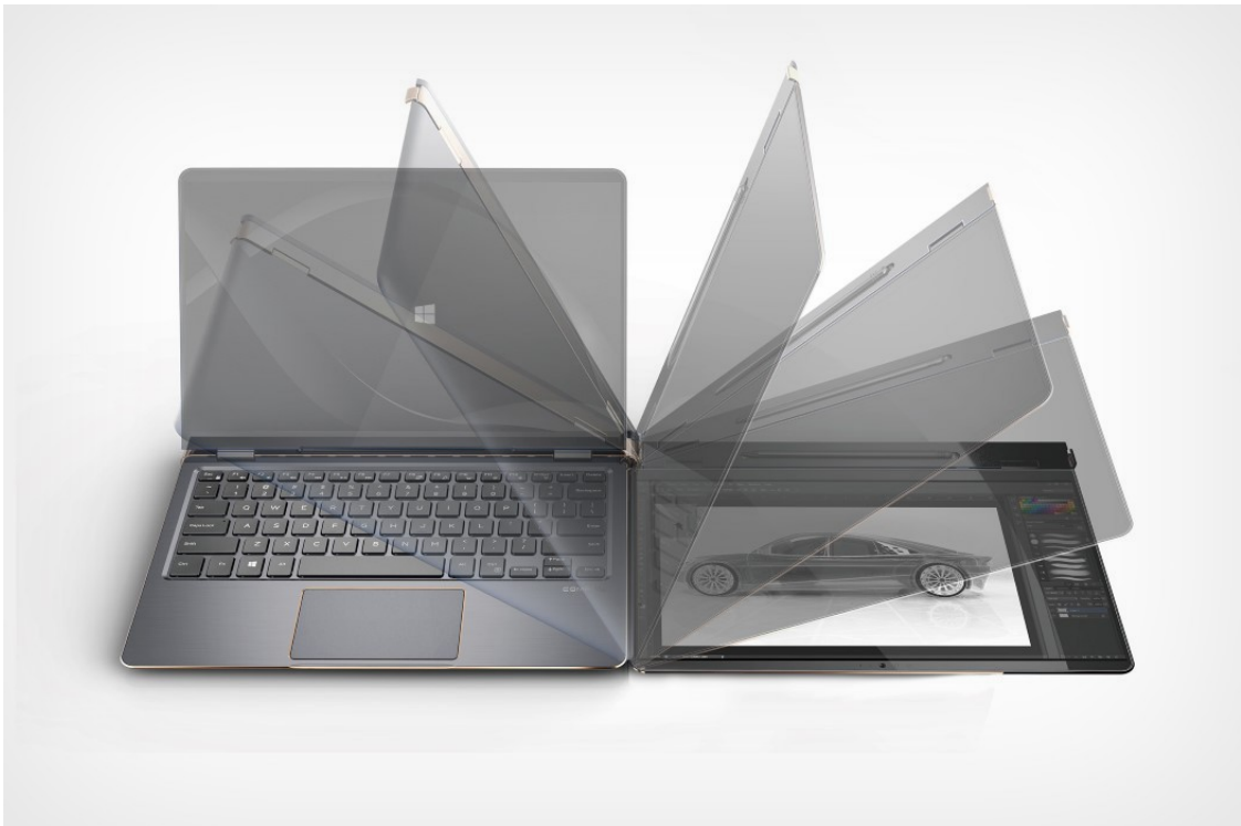
The DuoFlip( https://www.yankodesign.com/2019/03/29/the-duoflip-is-the-most-innovative-laptop-made-in-years/ ) opens in two ways, one like a traditional laptop with a backward hinge, and another, like a book with a hinge on the side by Compal Electronics( https://www.compal.com/ )
