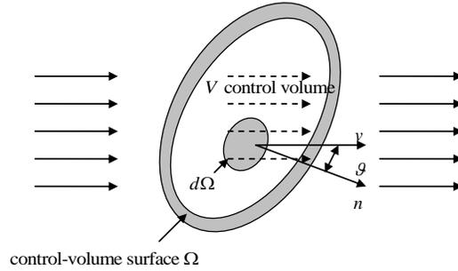
FIGURE 3. Control volume through which fluid flows
