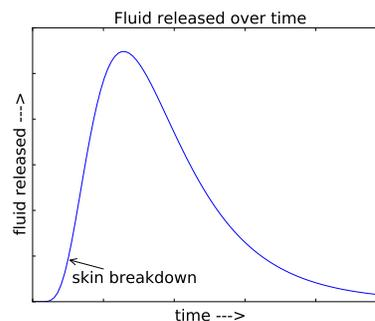
FIGURE 8. Amount of fluid released over time at constant temperature and ambient moisture
