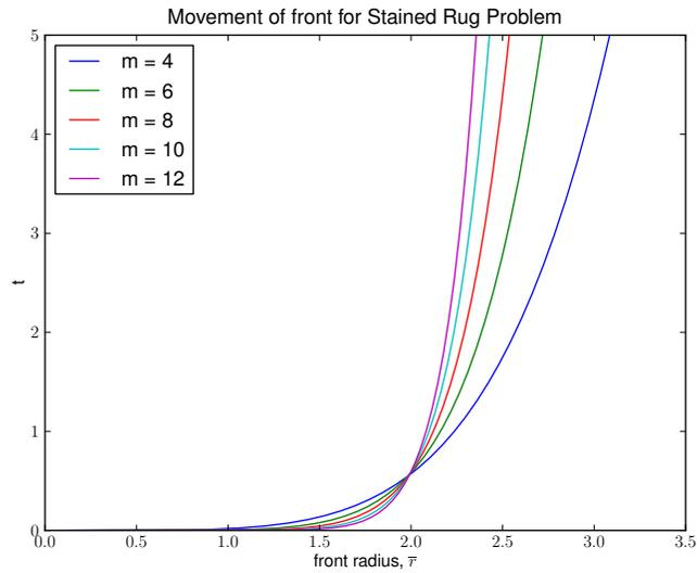
FIGURE 7. Evolution of the liquid front radius as a function of time
