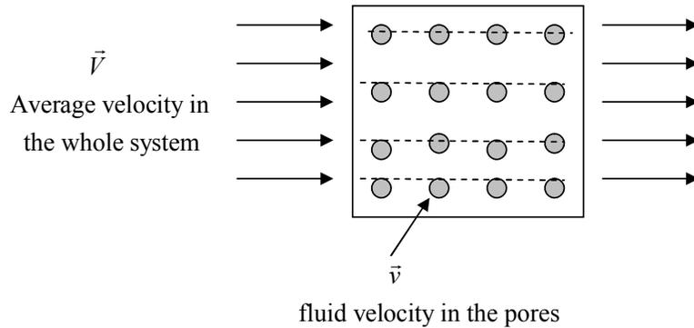
FIGURE 4. Fluid flow in porous media
