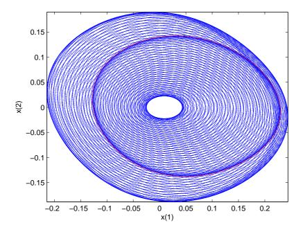
Figure 24: Computed torus of limit cycles curve started from a torus bifurcation of limit cycles
