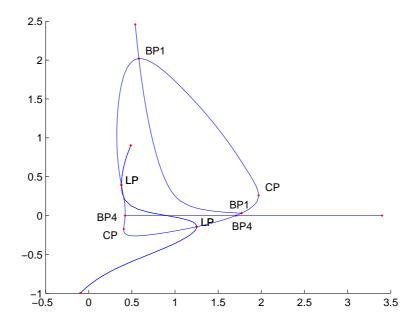
Figure 26: Computed BP curves started from Branch Points detected on a fold curve.
