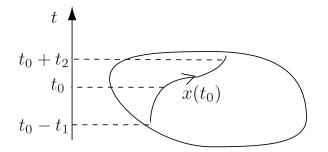
**Phase-space and flows**. Refer to local solution through  $x_0$  as a solution curve or trajectory. Suppose that  $\dot{x} = f(x)$ ,  $x \in \mathbb{R}^n$ ,  $f : \mathbb{R}^n \to \mathbb{R}^n$ . We define a flow  $\phi(x,t)$  such that  $\phi(x,t)$  is the solution of the ODE at time t with initial value  $x_0$  at t = 0. The solution x(t) with  $x(0) = x_0$  is now written as  $\phi(x_0, t)$
