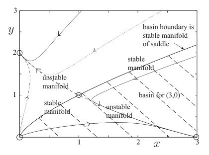
The above example nicely illustrates the notion of a **basin of attraction**. Given an attracting fixed point  $\overline{x}$  we define its basin of attraction to be the set of initial conditions  $x_0$  such that  $x(t) \to \overline{x}$  as  $t \to \infty$ . For instance the basin of attraction for the node at (3,0) consists of all points lying below the stable manifold of the saddle. Because the stable manifold separates the basins of two nodes, it is called the **basin boundary**.
