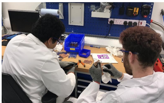
Preparing busbars for arc welding
