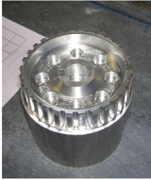
Figure 78 - Small Flipper Pulley Billet
