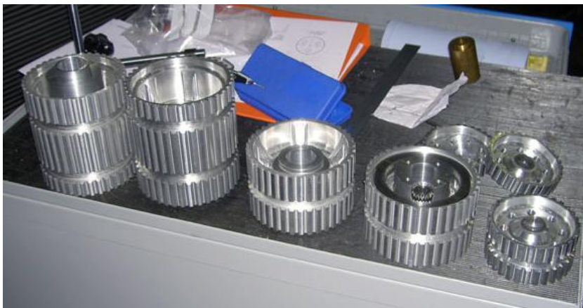
Figure 79 - Finish Machined Pulleys
