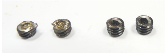
Figure 5-9: Sheared grub screws from the Parvalux gearbox output shaft
