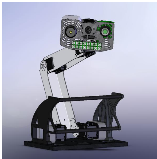
Figure 4-55: Arm in roll cage with servo mounting extensions visible
