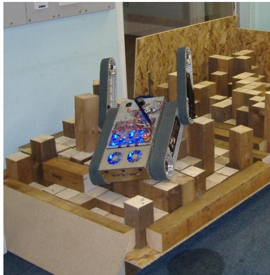
Figure 1-5: 2008 robot on a stepfield
