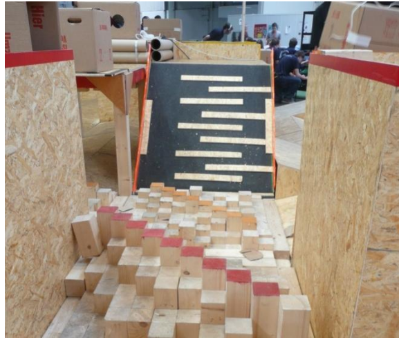
Figure 3-5: Stepfield run up to 45° ramp
