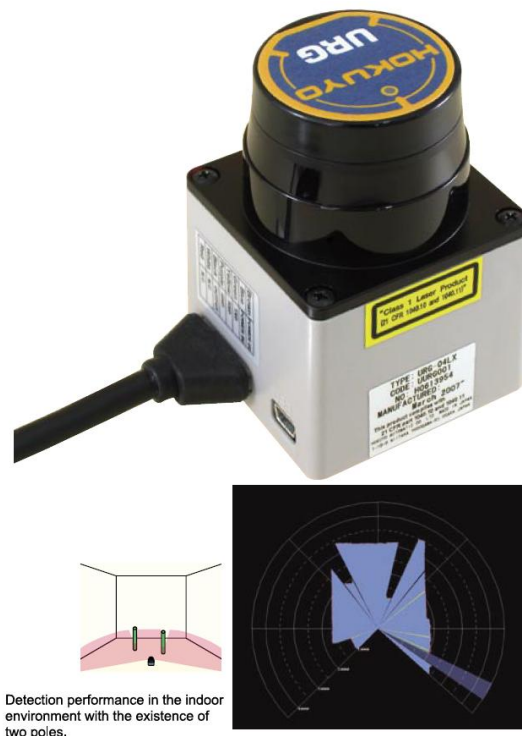
Figure 3-14: LiDAR unit for robot(6)
