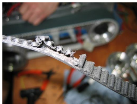
Figure 2-2: Typical flipper drive belt failure
