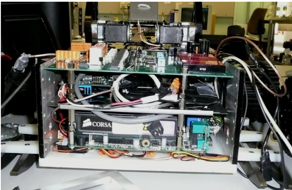
Figure 4-33: Central computer case mounted in the chassis
