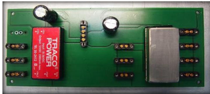
Figure 5: Final Power Distribution Board
