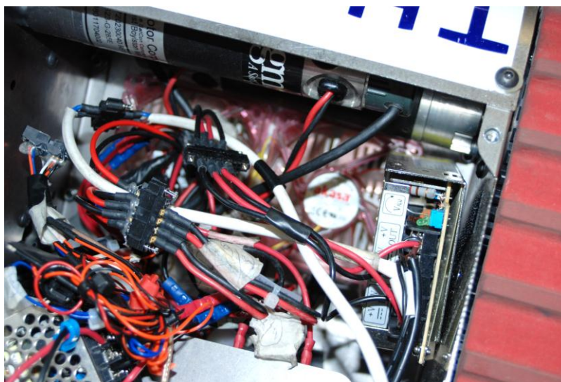
Figure 102: The connection of the 12V power converter to the chassis via velcro
