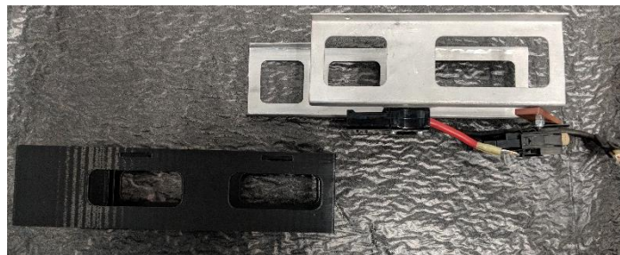
Figure 4.9: Two-part battery mounting system consisting of slider and mounting cage respectively.
