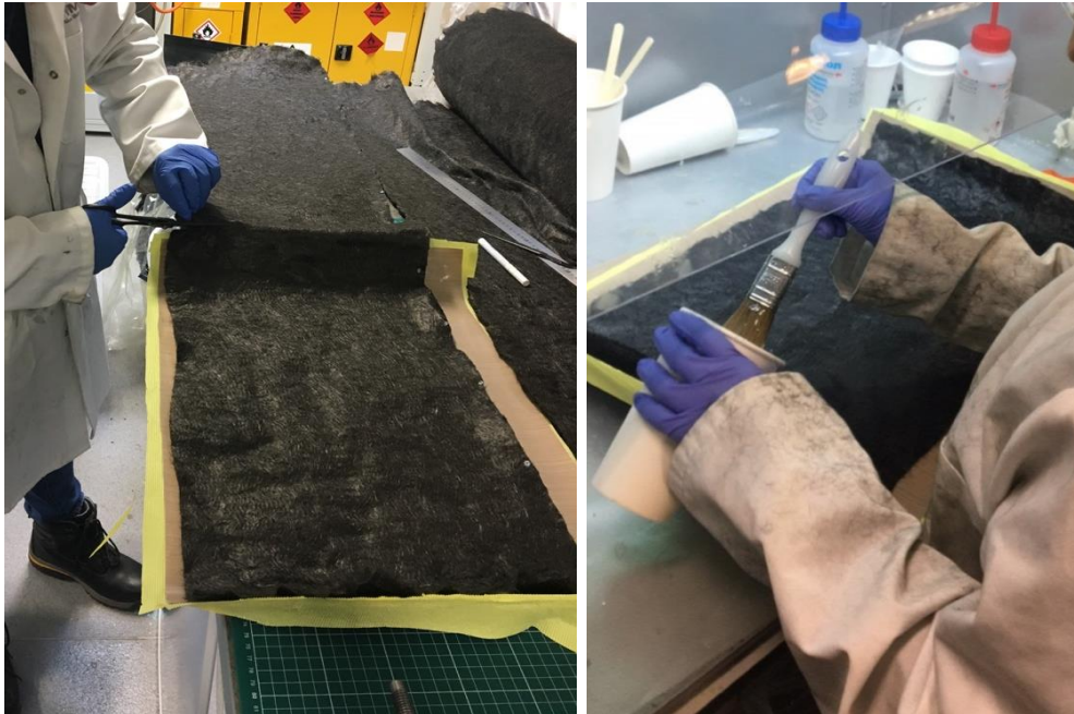
Figure 4.16: Cutting the carbon fibre matrix (left) and applying the resin (right)
