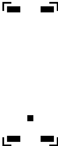
Layout of windows through protective photoresist to reveal electrodes and contact pads.
