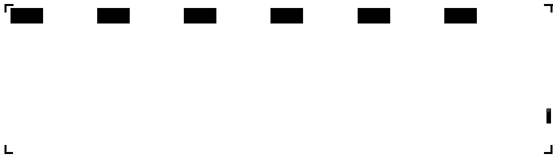
Layout of etch windows required in the \text{Si}_3\text{N}_4 thin film to expose the microheater contact pads.
