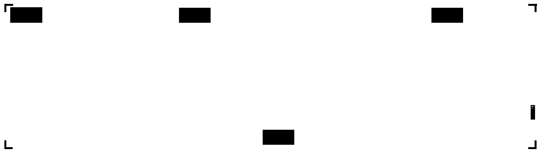
Layout of etch windows required in the thin film of Si 3 N 4 to expose the microheater contact pads.
