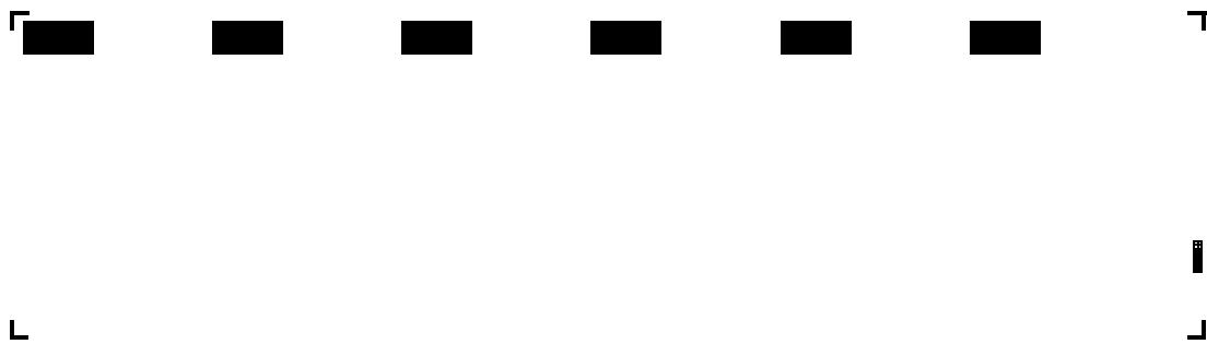
Layout of etch windows required in the thin film of \text{Si}_3\text{N}_4 to expose the microheater contact pads.
