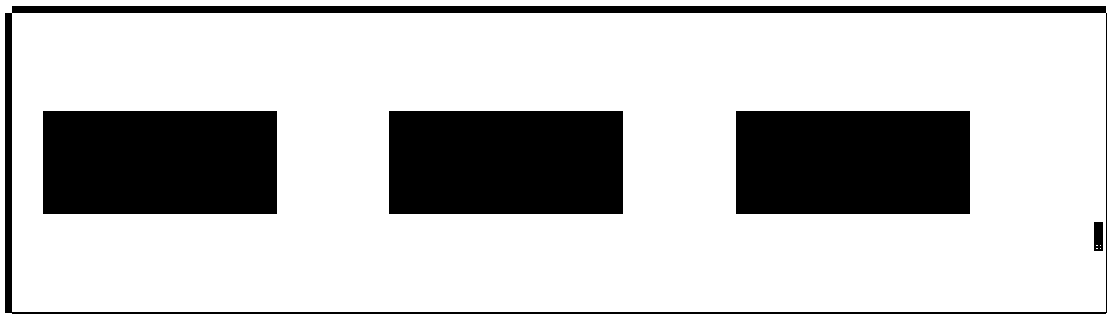
Layout of back-side KOH mask which defines the subsequent sensor structure after anisotropic etching.
