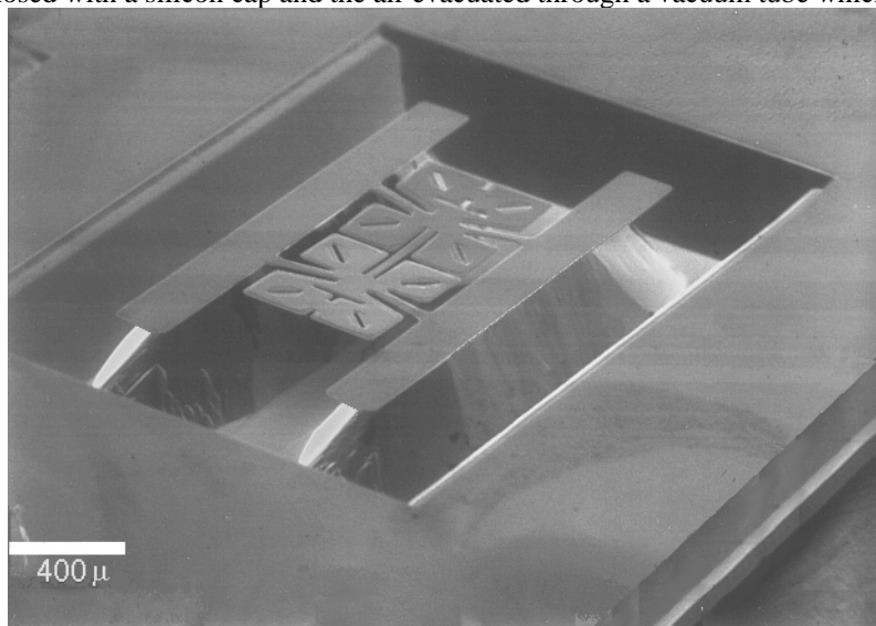
Figure 1.8 SEM showing the bulk micromachined resonant pressure sensor based upon a vibrating butterfly structure developed by Greenwood et al. This sensor is commercially available 4 .
