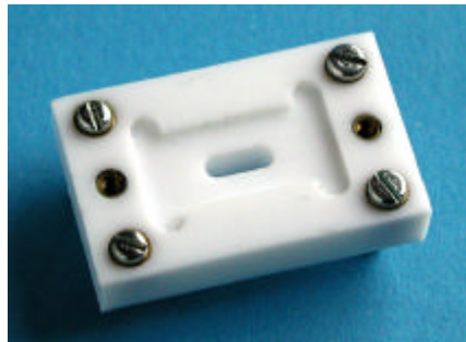
Figure 4.6 Picture of PTFE liquid cell with locating pins and central slot for liquid fill
