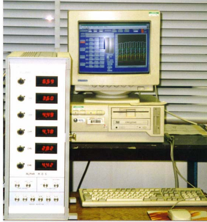
Fig. 3.4 Photograph of the Warwick Fox 2,000 electronic nose system.
