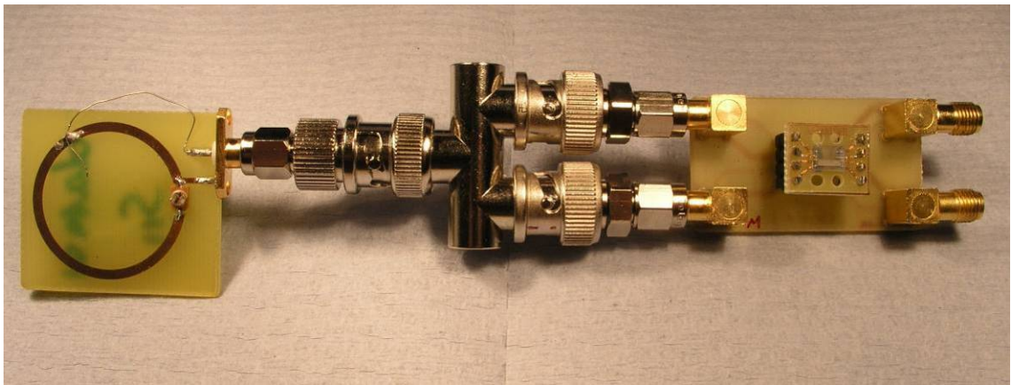
Figure 6.15: Loop antenna and test fixture for semi-wireless set-up
