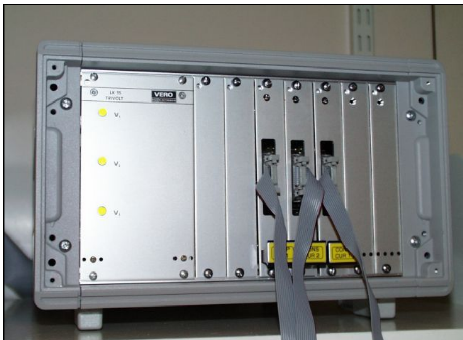
Figure 5.11: Constant current measurement instrument.
