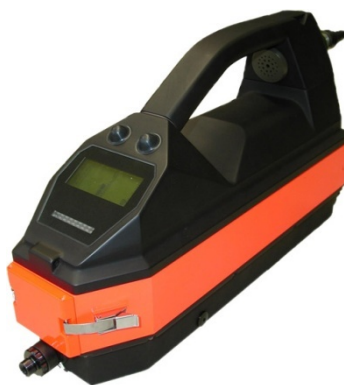
Figure 1.6 GDA 2 (Gas Detector Array 2) Portable detector for hazardous gases and chemical agents
