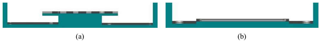
Figure 6.11: Microchannel package base designs for horizontal alignment. (a) Base design 1 (slot type). (b) Base design 2 (step type).
