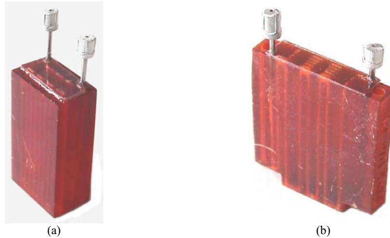
Figure 5.24: Complex microchannel packages with lid assembly. (a) MSL112 with plastic lid. (b) MSL113 with plastic lid.
