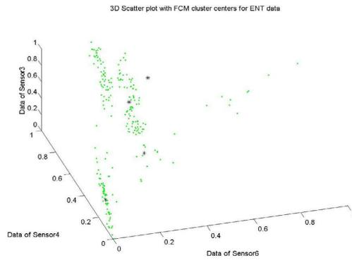
Figure 4: 3D view of the unsupervised FCM from non-conducting polymer sensor based Cyranó's e-nose.
