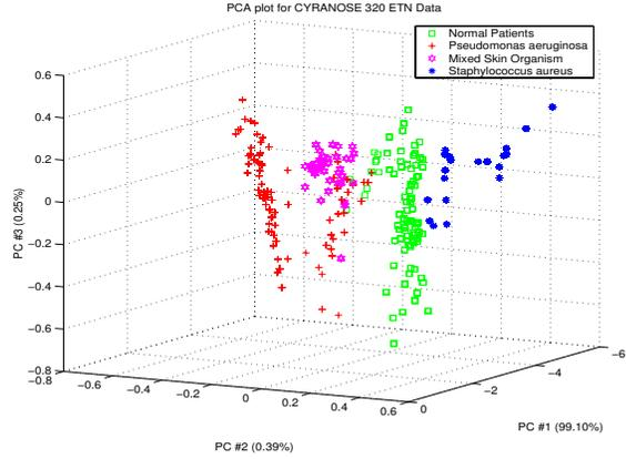
Figure 2: 3D view of the PCA plot for the e-nose data sets from four different ENT bacteria swab samples.
