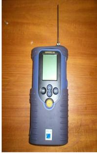
Figure 1: Typical Cyranose 320 e-nose
