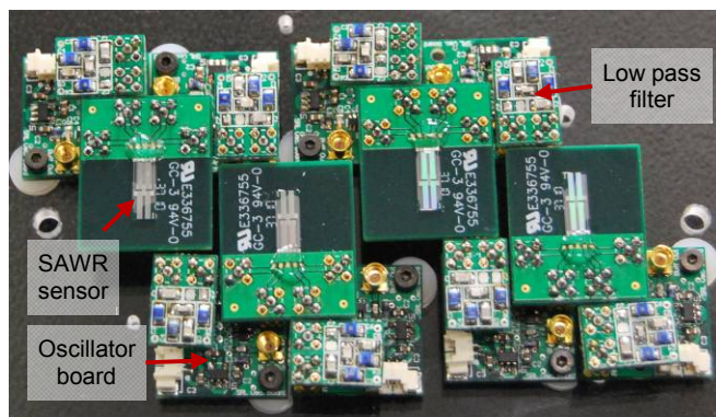
Figure 3. Photograph of a 4-sensor SAW resonator array with the associated radio-frequency oscillator circuits and low pass filters.
