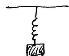
The system is modelled by the ODE  $\ddot{x}(t) = -kx(t)$  where  $x$  is the deviation from rest position and  $k$  is related to the weight of the mass of the object and the strength of the spring.
