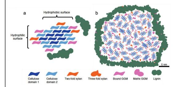
A possible model of the molecular architecture of softwood. a) A microfibril showing the two cellulose domains with 2-fold xylan and GGM bonded to the surfaces. b) A model of the macrofibril containing groups of cellulose microfibrils with bound GGM and xylan. Lignin is localised mainly to the surface of the macrofibril and interacts predominantly with GGM, xylan and cellulose domain 2
