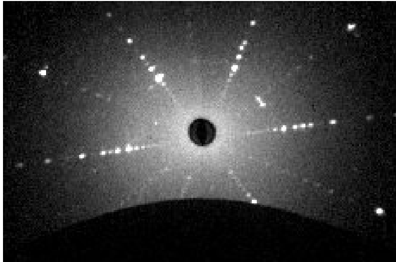
Figure 5.13: Laue backscattered reflection pattern along the [001] orientation of a \text{Cr}_{1/3}\text{TaS}_2 crystal.
