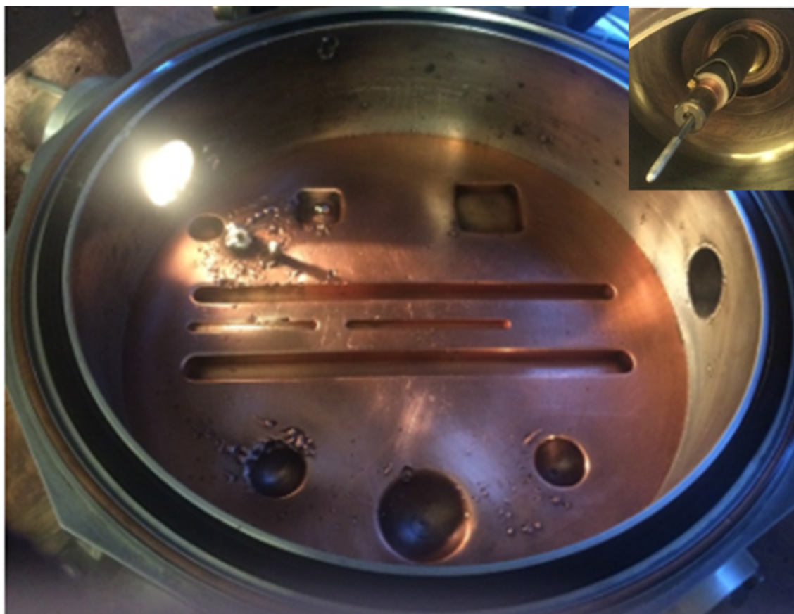
Figure 3.2: The crucible of the arc furnace. The arc is struck against the metal notch, as otherwise the large power output from the electrode causes it to fuse to the crucible. Inset: the electrode for the arc furnace.
