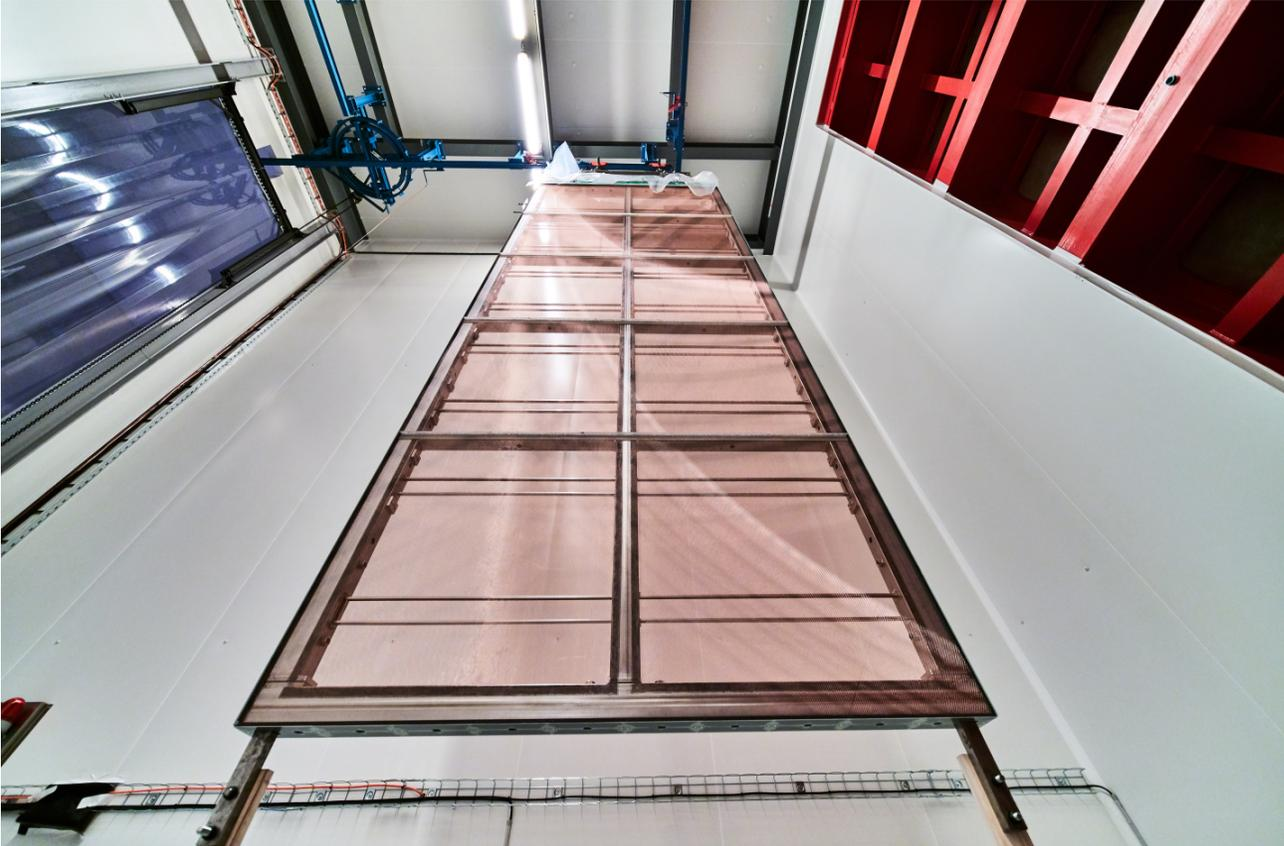
First APA ready to be installed in the protoDUNE-SP detector
