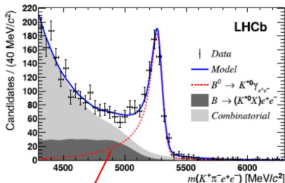
Long radiative tail in the B mass distribution: controlled from  $B \rightarrow K^* \gamma$  events ( $\gamma \rightarrow e^- e^+$ , with bremsstrahlung emission)
