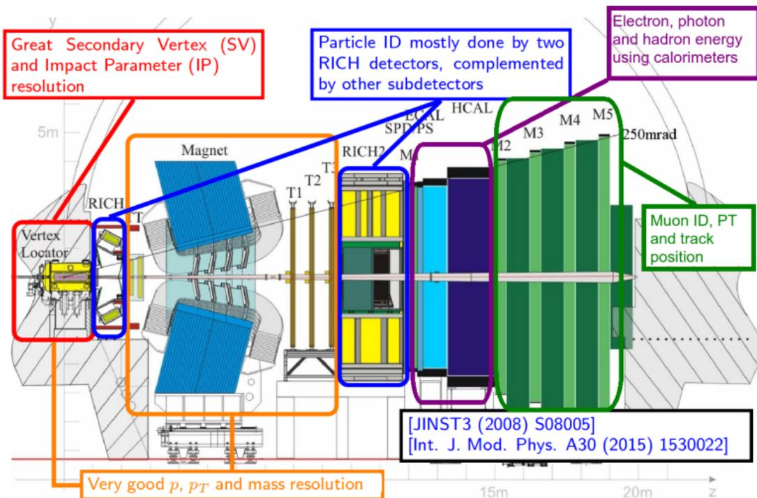
Muon ID  $\sim 97\%$  for  $\sim 1\text{-}3\% \pi \rightarrow \mu$  mis-id probability
