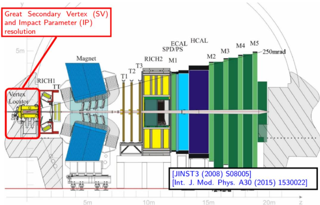
$$\Delta IP = (16 + 29/p_T [\text{GeV}]) \mu\text{m}$$
