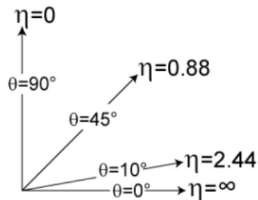
$\theta$ : Angle between  $\mathbf{p}$  and positive beam axis.
