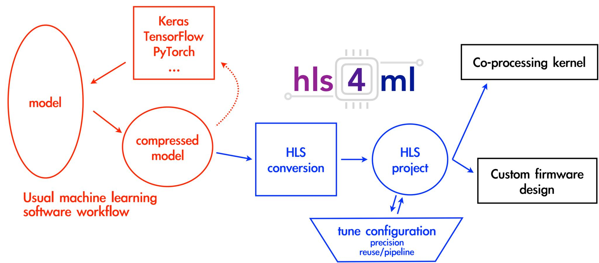
**HLS** - High Level Synthesis - compiler for C, C++, SystemC into FPGA IP cores
