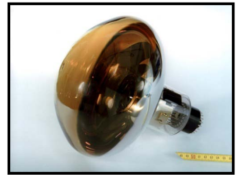
Hamamatsu PMT : Size :10 inch
