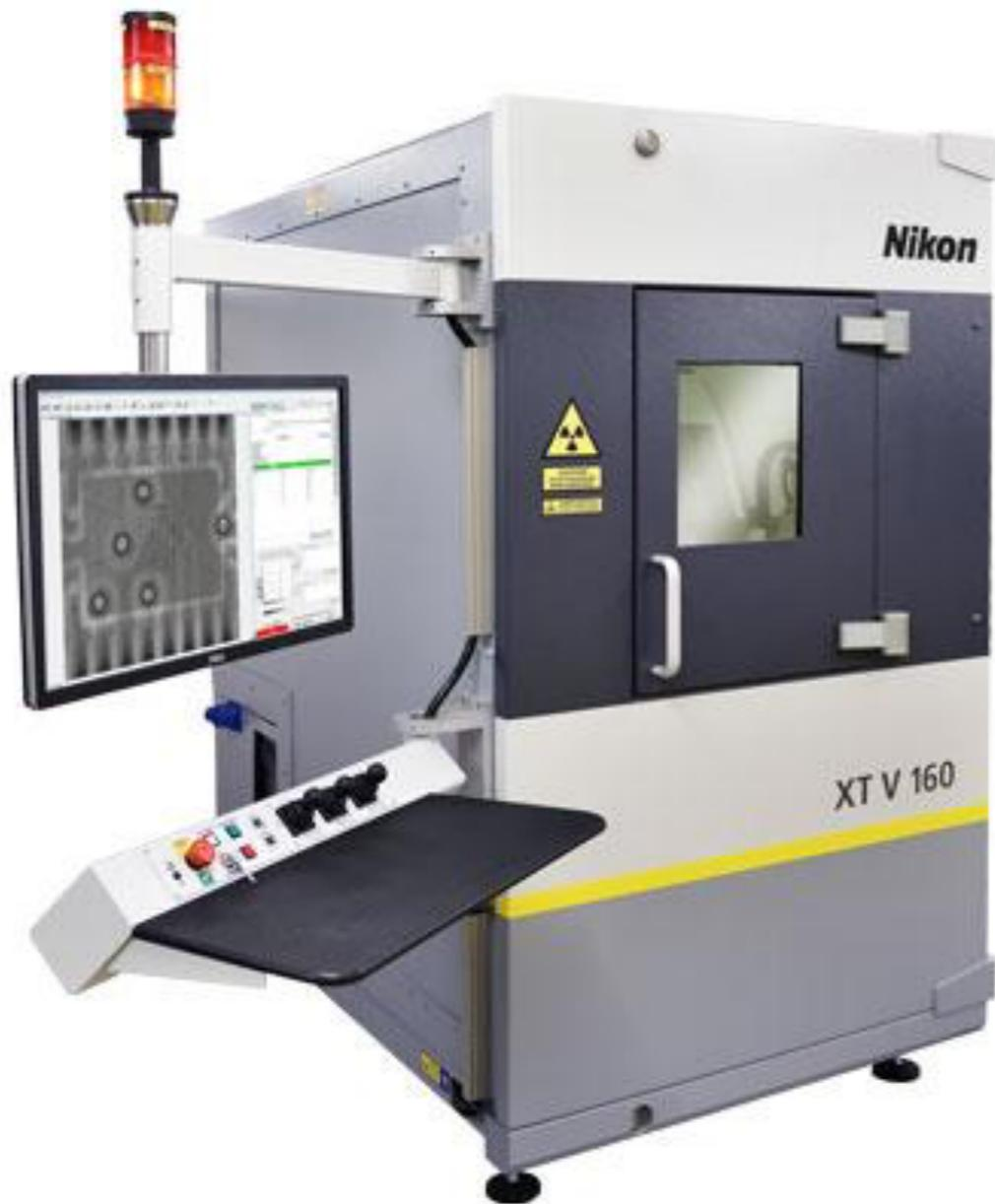
X-ray Computed Tomography (CT) is a nondestructive technique for visualising interior features within solid objects, and for obtaining digital information on their 3-D geometries and properties.
